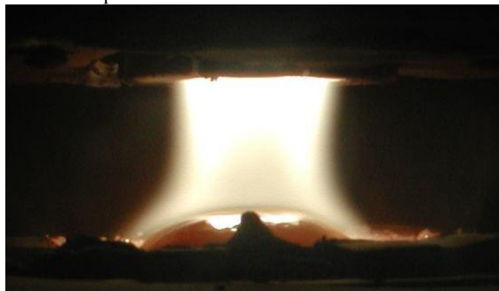
Figure 2: Liquid silicon dome under plasma.
