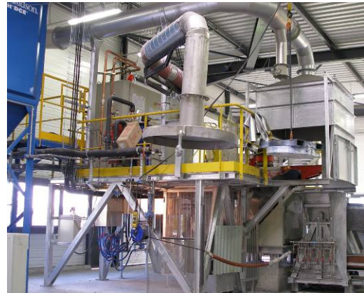
Figure 3: Outside view of the segregation equipment for the production of UMG-2 Silicon.
