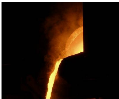
Figure 2: Transfer of melted Si into segregation vessel
