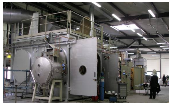
Figure 4: Outside view of the plasma purification and solidification unit.
