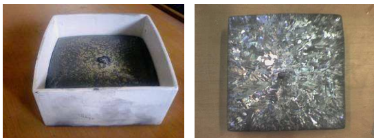
Figure 4: 6kg ingot from doped electronic grade Silicon, inside the crucible (left) and after chemical cleaning (right).
