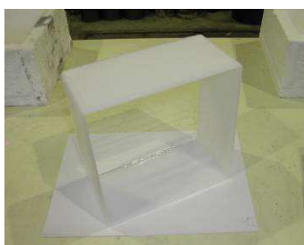
Figure 4: Photo of a 200x200x100mm 3 anisotropic quartz crucible with transparent bottom and opaque side walls.
