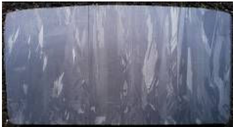
Figure 4 : Vertical grain structures on a vertical cut from a multi-crystalline Silicon ingot
