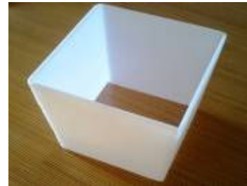
Figure 3: Photo of an anisotropic quartz crucible with transparent bottom and opaque side walls.
