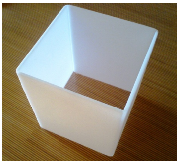
Figure 3: Anisotropic quartz crucible 200x200x220 mm 3 for 12 kg ingots.
