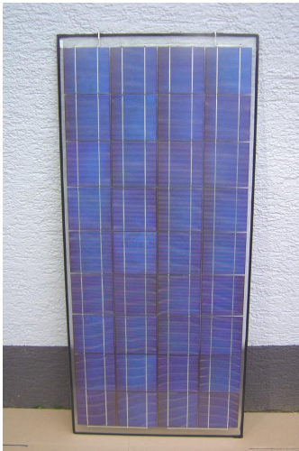
Figure 4: One of the first 36 cells modules realized with multi-c solar cells and textured extra white glass sheets.
