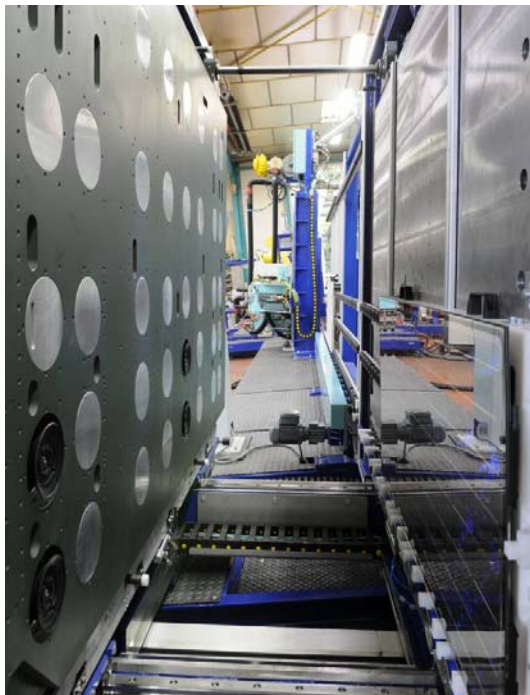
Figure 7: Module Press for the flooding with neutral gas, establishing the under pressure and the assembling of rear and front sheets.
