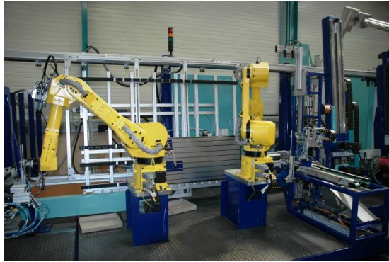
Figure 6: Cells and Ribbons deposition station with unrolling, straightening, forming and cutting of copper ribbons serving as metal interconnectors.
