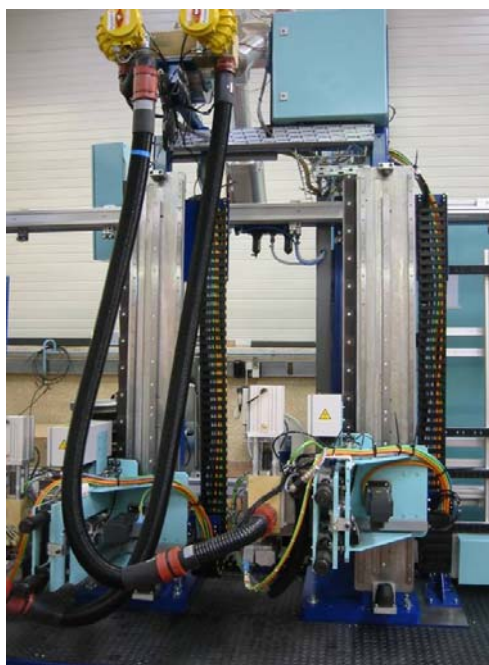
Figure 5: PIP sealing deposition unit: Two nozzles are in place, one for the deposition of gluing stripes for the fixation of the different components (cells, ribbons, module busbars and external connectors), the other nozzle for the sealing line on the perimeter of the module.
