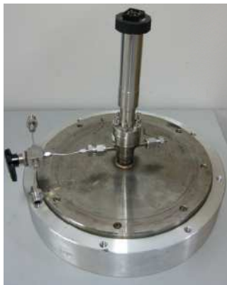
Figure 4: Modified set up for air leakage tests
