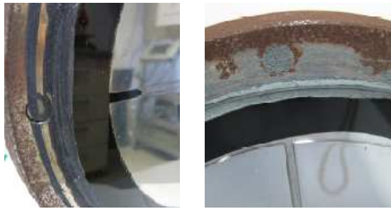
Figure 7: PIB that has migrated into the groove due to non sufficient adhesion (left) and PIB that adhered perfectly (right).
