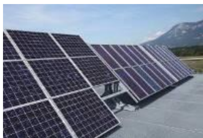
Figure 7: Laminated modules and NICE modules under outdoor exposure
