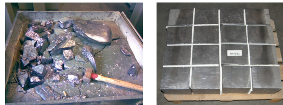
Figure 3: Pictures of plasma purified silicon rapidly solidified (left) or in a directionally way (right).
