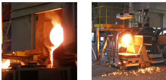
Figure 1: Pictures showing the transfer of the melted silicon in the segregation vessel (left) and the elimination of the impurities enriched silicon (right).
