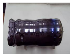
Figure 7: Picture of the 6" Cz monocrystalline ingot made from 100% of the highly purified PHOTOSIL silicon.
